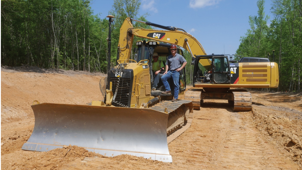
Vice President of Wellons Construction, Seth Thompson, with Topcon equipment. Shown in image is Topcon 3D-MC 2 GPS system installed with Caterpillar dozer and Topcon X-53i on Caterpillar excavator.
